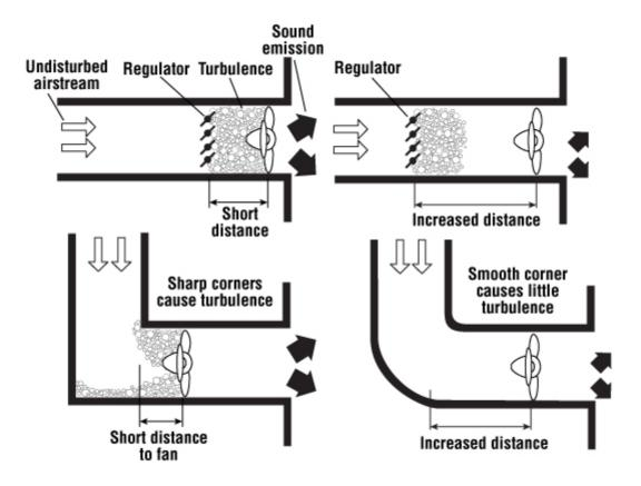
Figure 1: How to avoid turbulence (Figure from: World Health Organization, (1996). "Engineering Noise Control")
