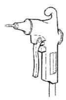
Select hand tools that encourage a good grip, such as non-slip, non-conductive and compressible materials like plastics or compound rubbers. The goal is to reduce the effort needed to use the tool effectively and at the same time, prevent the tool from slipping out of the hand.
