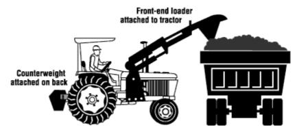
• Remove the loader from the tractor when not in use, if possible.
